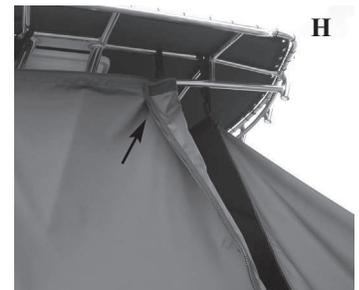
Take the larger section of the cover and place the portion that contains the draw rope over the starboard side rub rail. Position the remaining section of the cover over the motor or motors. Find the stern half of the zipper and join to the forward half of the zipper located between the console and helm seat zipping approximately one third of the way.
