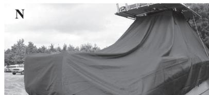
Improperly Installed Cover
