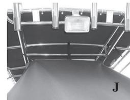
④ Depending on the size of your T-top cover, there may be additional straps to secure. If so, continue connecting the remaining straps in a counter clockwise motion to any horizontal bar found under the canvas top. While stepping out of the boat complete zipping the remaining portion of the zipper. At the bottom of the zipper is a draw rope which has loops on both ends. Slide one end of the rope through a loop and draw the rope tight. Make a clove hitch knot at the end of rope. (See photos K-M.)
