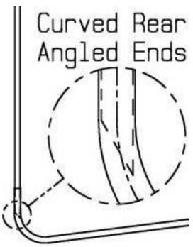
is pushed in as far as possible on both sides. It should measure 50" across the outside at the back when properly assembled. If it is 52" or more wide (to the outside), then you have the Curved-Rear-Cross-Bar in backwards, and you must take it apart and flip it around.
