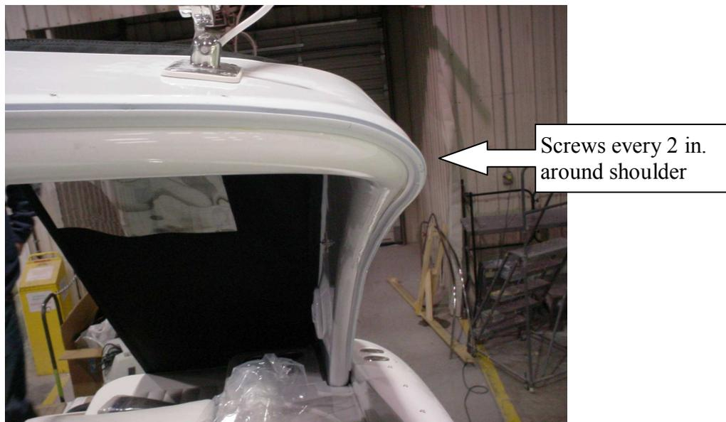
9. Use a 35” piece of track to continue the installation to bottom of the exposed arch.
