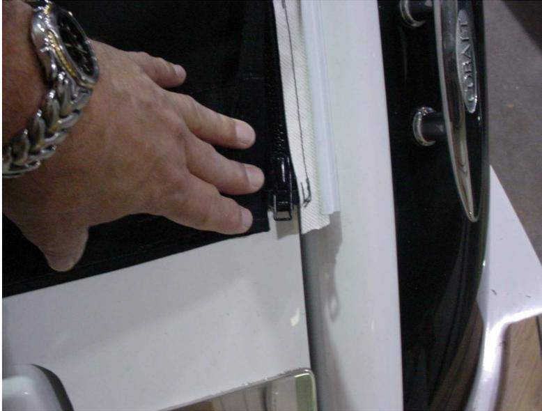
13. Caulk seam between arch and track with silicone caulk. Run a very thin bead, wet with soapy water, and smooth with finger.
