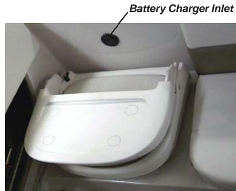
**Figure H3: Fish & Ski Built-In Battery Charger Inlet**
