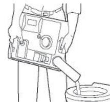
Figure J10: Emptying Waste Holding Tank
