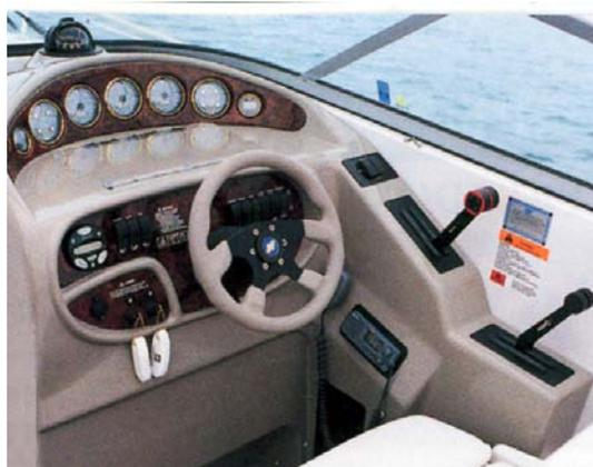
Figure E4: Helm Station - Twin Engine
