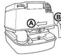
Figure J9: Removing Fresh Water Tank
