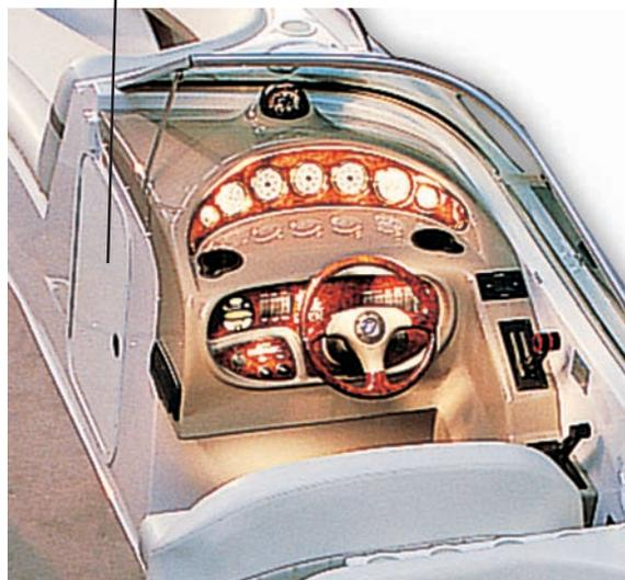
Figure L12: Walk-Thru Helm Console Storage
