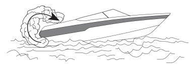
Figure 2.4 Exhaust Accumulation due to High Bow Angle or Slow Speed
