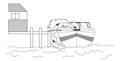
Figure 2.1 Running engine or generator in confined areas
