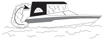
Figure 2.3 Exhaust Accumulation While Canvas is in Place
