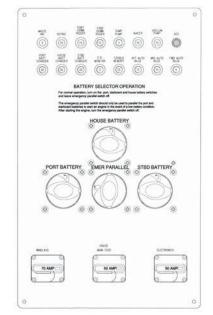
Figure 3.1 Four Selector Switches with Three Batteries and Twin Engines
