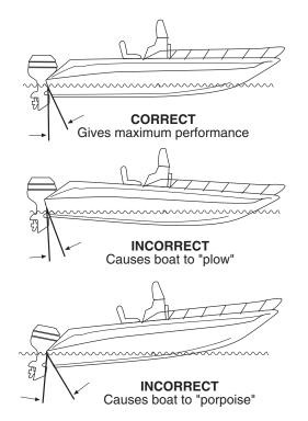
Figure 5.3 Trimming the Drive Angle
