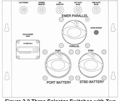
Figure 3.2 Three Selector Switches with Two Batteries and Twin Engines
