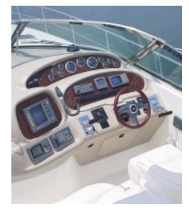
At the helm, the captain enjoys a wood-accent tilt wheel with hydraulic steering and dual gear shift and throttle controls.
