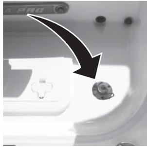
The intake seacock/pump supplies seawater to the deck fitting. The fitting allows for connection of a common garden hose and there is a cap that is tethered to the fitting which should be **ON THE CONNECTION** when it is not in use.
